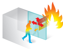
EW 'Integrity and Radiation Limitation': Restricts heat transfer to no more than 15kW/m 2
