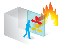
EI 'Integrity and Insulation': Blocks heat transfer
